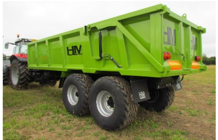
Paul’s new trailers have a 22 tonne running gear, heavy duty axles and will be easier to back up to the hopper, meaning less damage and loss. With all three trailers being the same spec and height, Paul will be able to set the hopper to the same height and use multiple trailers without having to re-set the hopper, saving time and labour.
